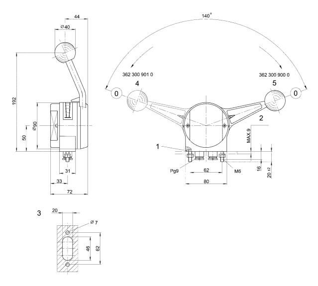
1) Seal, 2) Mounting plate, 3) Cutout of mounting plate, 4) Left-hand version, 5) Right-hand version Assembly position is open
