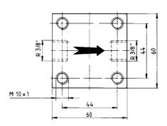
Assembly position as drawn. Space for dismounting of container and draining of condensate (screw 1) has to be available.
