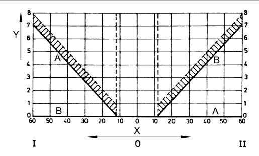
x) Lever travel [°], y) Pressure in port A [bar] In area 0 - I pressure A in valve 2 = 0 bar, in area 0 - II pressure A in valve 1 = 0 bar
