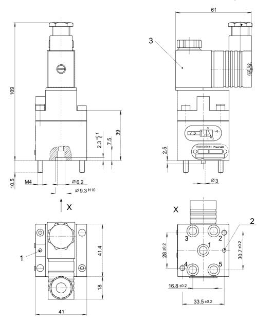
1) Check pin (reeled-out if pressure in connection 1 >4 bar), 2) Dowel pin , 3) Solenoid can be turned by 90°.
