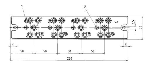
1) Thread for valve mounting, 2) Hole for dowel pin
