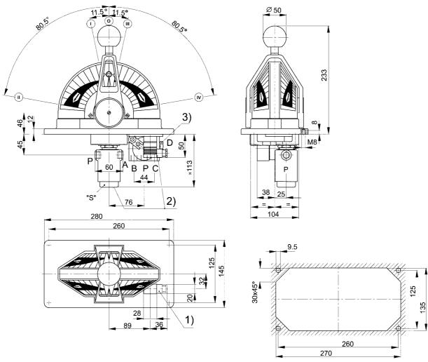
1) Device plug, 2) Exhaust, 3) Plug screw
