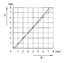
x) Input pressure p4, y) Outlet pressure p2
