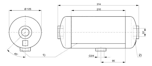
1) Longitudinal seam, 2) Container shield
