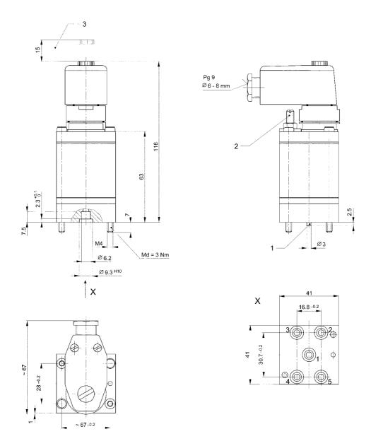
1) Dowel pin, 2) Adjusting screw for switching pressure, 3) Space to take out the connector
