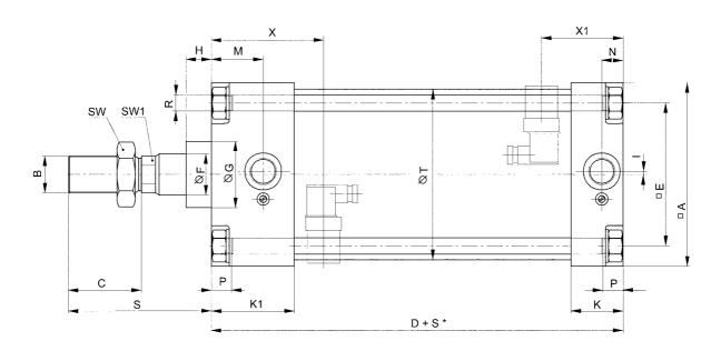
$S^*$  = Stroke, x) Position of the solenoid, extracted x1) Position of the solenoid, returned For standard cylinders of 250 mm dia. the tie rods protrude by 45 mm from the cylinder's top and bottom covers.
