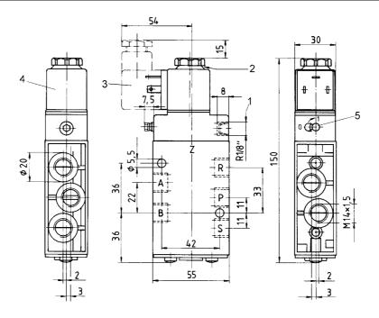
1) Only with separate pilot control G 1/8 2) After removal of cap internal thread M5 3) Plug can be fixed at 180° intervals 4) Coil can be fixed at 45° intervals 5) Manual override
