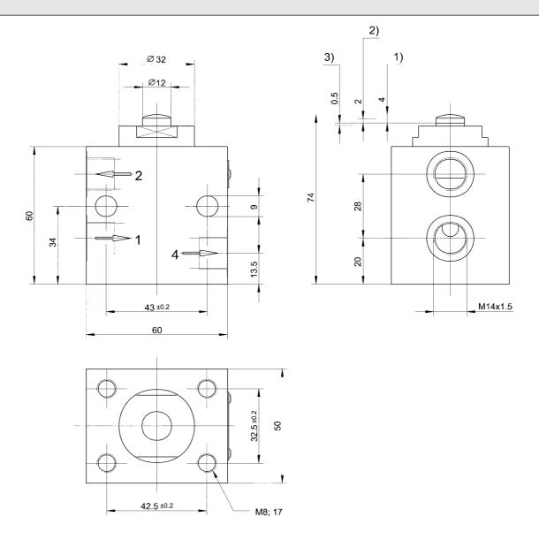
1) Stroke, 2) Ventilation resp. exhaust stroke, 3) Excess stroke
