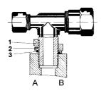
1) Lock nut, 2) Thrust ring, 3) O-ring
