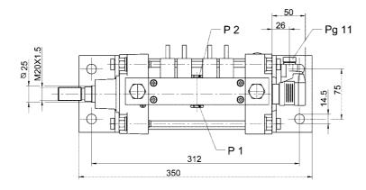
Installation: Valves' positions preferably vertically upright. Admissible deviation of up to  $90^{\circ}$  in each direction.
