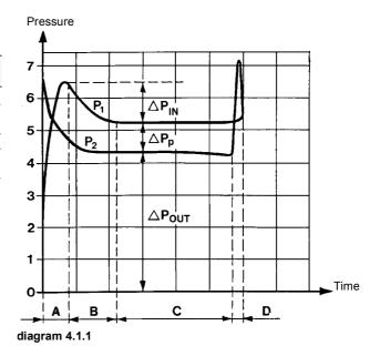
A Starting time C Steady state B Acceleration D Cushioning
