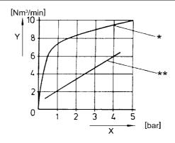
x) Pressure drop, y) Flow rate, \*) NC-valve, \*\*) NO-valve
