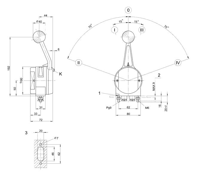
K) Speed increase-Gear interlock, 1) Seal, 2) Mounting plate, 3) Cutout of mounting plate Assembly position is open
