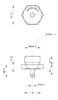
The valve has to be screwed in the end-plate connection of the container and sealed with sealing ring 810 401 079 4.
