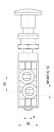
Assembly position is open Control panel bore diameter 23 mm
