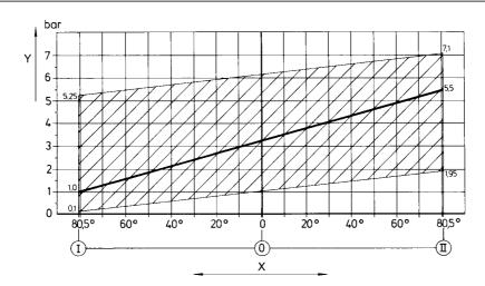
The characteristic line is infinitely adjustable in an parallel way within the shaded area and its gradient can be modified. Observe, that the pressure difference between initial and final pressure must be more than 1.85 bar. X) Handle travel, Y) Pressure in connection A
