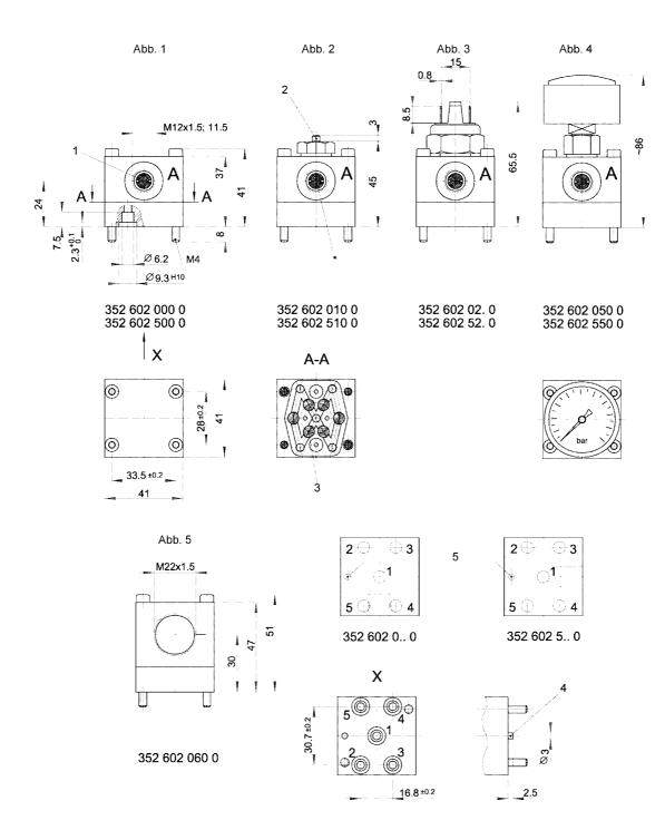
1) Strainer, 2) Check pin, 3) Plug, 4) Dowel pin, 5) Dowel pin and position of threaded connection
