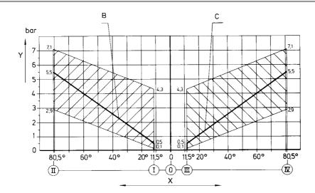
The characteristic line is infinitely adjustable in an parallel way within the shaded area and its gradient can be modified. Observe, that the pressure difference between initial and final pressure must be more than 1.85 bar. X) Handle travel, Y) Pressure, B, C) Connections
