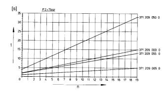
t) Time delay, n) Number of rotations of the adjusting screw
