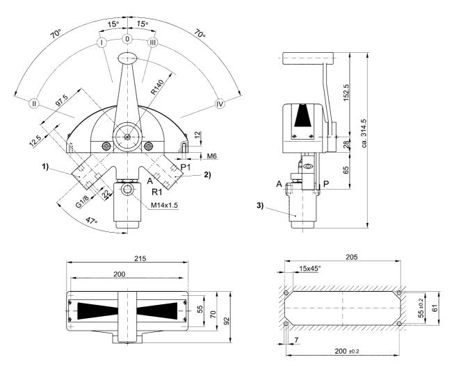
1) Valve 1, 2) Valve 2, 3) Pressure regulating valve
