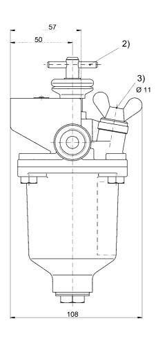
Assembly position vertically as drawn. Space for topping-up antifreeze and activating the toggle handle has to be available.
