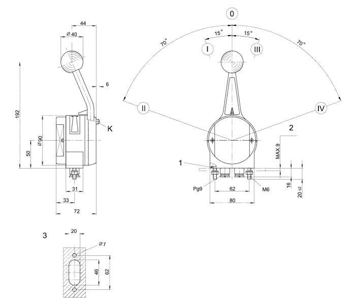
K) Speed increase - Gear interlock, 1) Seal, 2) Mounting plate, 3) Cutout of mounting plate Assembly position is open
