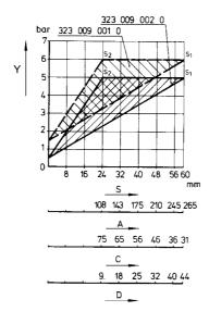
S1 = Longest travel, S2 = Shortest travel, y = Pressure in connection 1 S = Travel, A = Rod length, C = Length C, D = Length D
