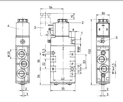
1) Only with separate pilot control G 1/8 2) After removal of cap M5 internal thread 3) Plug can be fixed at 180° intervals 4) Coil can be fixed at 45° intervals 5) Manual override
