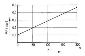
The actuator's hysteresis is decisively influenced by friction forces at the actuation mechanism of the device to be operated. x = Force (friction forces) at piston rod
