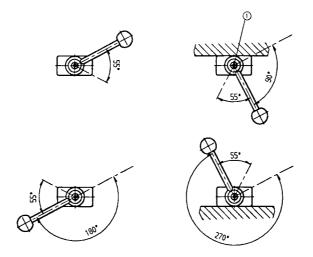
1) Loosen the screw to adjust the initial position
