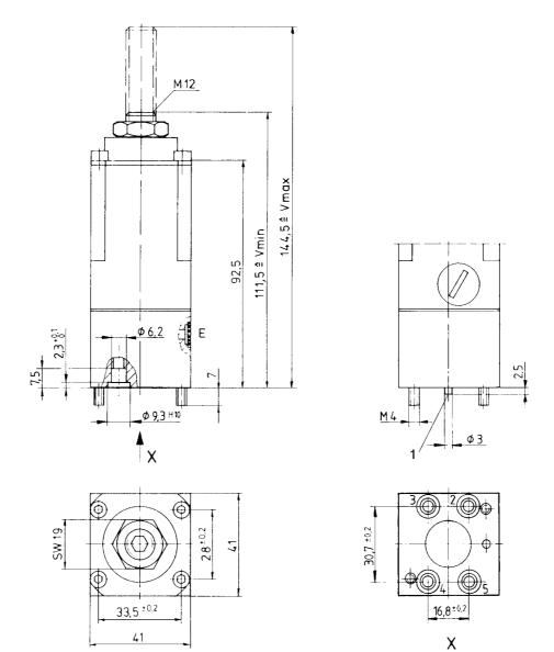
1) Dowel pin Close off unused connections with the enclosed seals 897 110 670 4 or 897 678 4.
