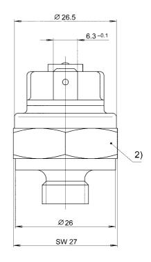
1) Sealing surface 2) Change-over pressure and type of switch are stamped.
