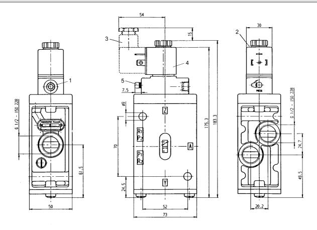
1) Only with separate pilot control G 1/8 2) After removal of cap internal thread M5 3) Plug can be fixed at 180° intervals 4) Coil can be fixed at 45° intervals 5) Manual override
