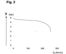
Fig.1 Pressure travel characteristic line x: Regulating stroke [mm] y: Pressure at port A [bar] a: Characteristic line b: Exhaust stroke Example: regulating range 0.1 - 5.1 bar V = max. parallel shifting: 1.4 bar Fig. 2 Nominal flow rate Input pressure: 8 bar; supply pressure: 6 bar y: Pressure at port A [bar]
