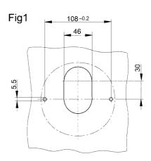
S) Adjusting screw Fig. 1 Cutout of panel mounting
