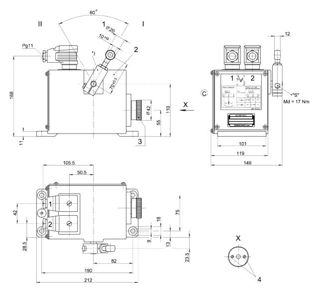
1) Ball 2) Adjustable from 60 mm to 75 mm 3) Hand-wheel operator 4) Adjusting screws for automatic locking \*) After loosening the screw S the lever can be adjusted in any position.
