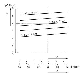
X) Trip point pressure, A) Rotations at adjusting screw, Y) Reset pressure, B) Final control adjustment Trip point pressure can be changed by ±0.3 bar by means of the adjusting screw. In this way also the reset pressure will be changed.
