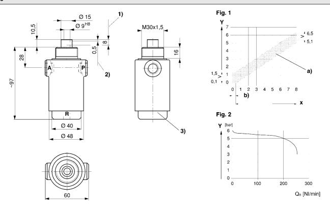
1) Stroke 2) Closing or exhaust stroke 3) Screw cap
