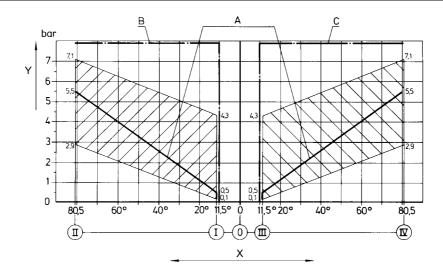
The characteristic line is infinitely adjustable in an parallel way within the shaded area and its gradient can be modified. Observe, that the pressure difference between initial and final pressure must be more than 1.85 bar. A, B, C) Connections, X) Actuating angle, Y) Pressure
