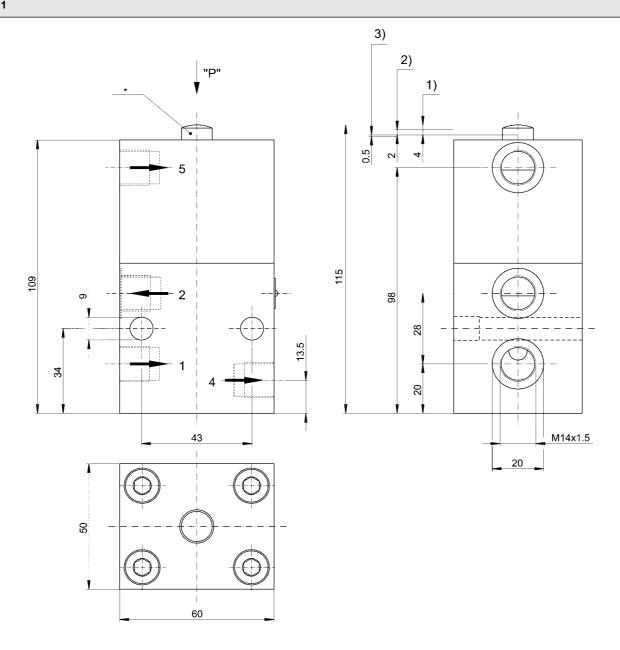
1) Stroke, 2) Ventilation resp. exhaust stroke, 3) Excess stroke \*) Emergency operator
