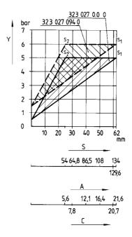
y = Pressure in connection 1, S = Travel, A = Rod length A, C = Length C
