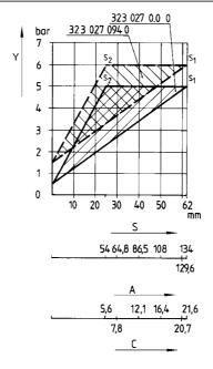
y = Pressure in connection 1, S = Travel, A = Rod length A, C = Length C
