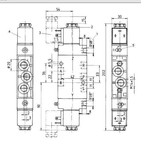
1) Only with separate pilot control G 1/8 2) After remova 4) Coil can be fixed at 45° intervals 5) Manual override 2) After removal of cap M5 internal thread 3) Plug can be fixed at 180° intervals
