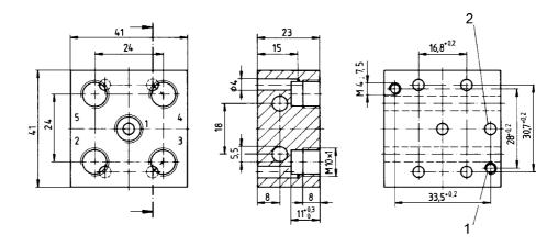
1) Thread for valve mounting, 2) Hole for dowel pin
