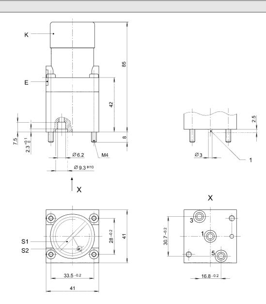
K) Protective cap, E) Exhaust, S1) Adjusting screw, S2) Safety screw, 1) Dowel pin
