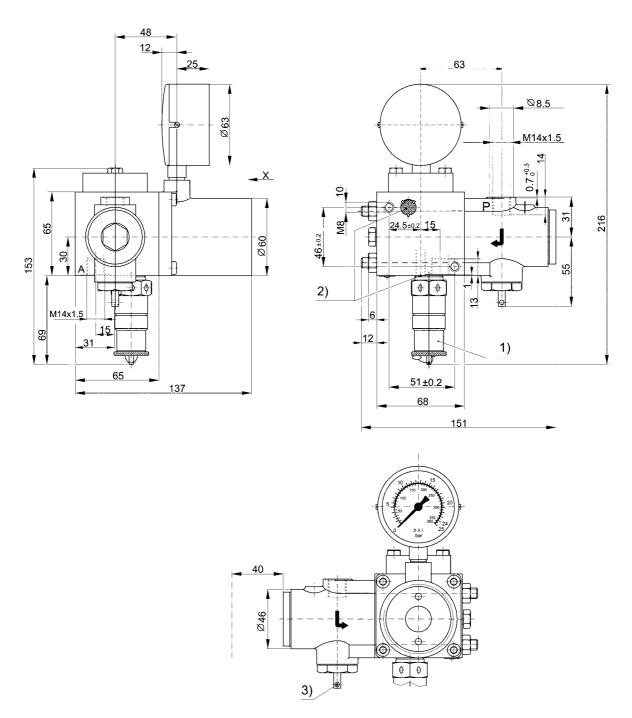
The device has to be mounted vertically as shown. Admissible deviation  $\pm 45^\circ$  to drawn position. 1) Safety valve, 2) Exhaust, 3) Drain valve
