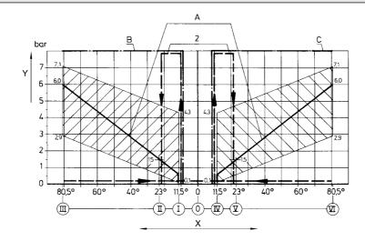
The characteristic line is infinitely adjustable in an parallel way within the shaded area and its gradient can be modified. Observe, that the pressure difference between initial and final pressure must be more than 1.85 bar. X) Handle travel, Y) Pressure, A, B, C, 2) Connections
