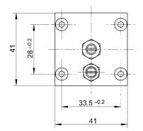
1) Dowel pin Close off unused connections with the enclosed seals 897 110 670 4 or 897 678 4.
