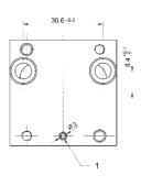
1) Dowel pin, 2) Throttle adjustment
