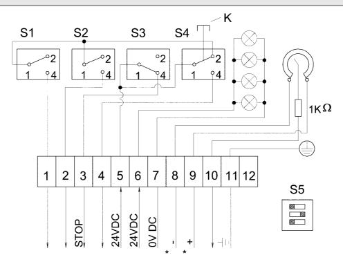
Speed increase / Gear interlock (warming-up function): by pressing button K and moving the lever over STOP in direction AHEAD or ASTERN the engine speed will be increased without engaging the clutch. When moving the lever back to STOP-position the gear function will be automatically active again. ATTENTION: Note switch C in the connection diagram! \*) Stabilized voltage
