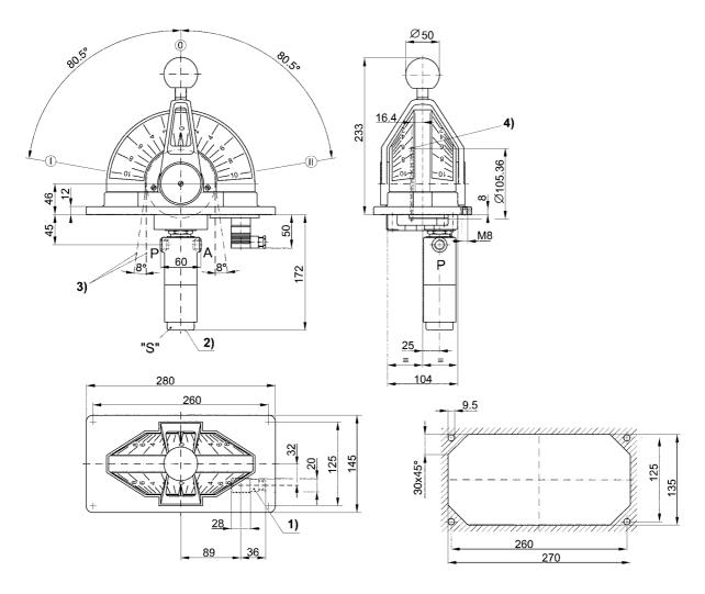
1) Device plug, 2) Exhaust, 3) Max. range for chain guide, 4) Sprocket wheel (z=26, t=12.7) suitable for chain 083 DIN 8187
