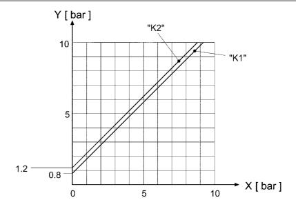
x) Control pressure p5, y) Working pressure p2
