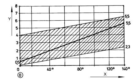
The characteristic line is infinitely adjustable in a parallel way within the shaded area, and its gradient can be modified. Observe that the pressure difference between initial and final pressure must be more than 2.2 bar.
