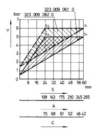
y = Pressure in connection 1, S = Travel, A = Rod length A, C = Length C
