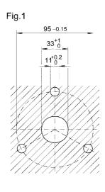
4) Adjusting wheel for increase (do not adjust under pressure) - Anti-clockwise rotation = higher characteristic line 5) Adjusting wheel for parallel shifting of characteristic line - clockwise rotation = higher pressure Fig. 1 Cutout of panel mounting
