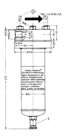
Assembly position as drawn. Space for dismounting of container and draining of condensate has to be available.
