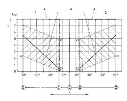
The characteristic line is infinitely adjustable in an parallel way within the shaded area and its gradient can be modified. Observe, that the pressure difference between initial and final pressure must be more than 2.2 bar. X) Handle travel, Y) Pressure in connection A, 1, 2) Valves 1 and 2
