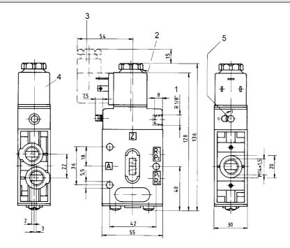
1) Only with separate pilot control G 1/8 2) After removal of cap M5 internal thread 3) Plug can be fixed at 180° intervals 4) Coil can be fixed at 45° intervals 5) Manual override
