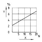
The actuator's hysteresis is decisively influenced by friction forces at the actuation mechanism of the device to be operated. y = Hysteresis, x = Friction
