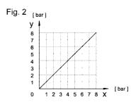
Fig. 1 Cutout of panel mounting Fig. 2  $\,$  x: pressure in control line 12  $\,$  y: pressure in working line 2
