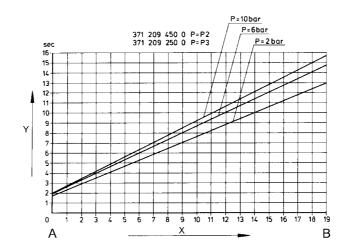
x) Number of rotations, y) Time, A) Min. volume, B) Max. volume The diagram is valid for P1 = P2. For longer switching times an additional volume in in port 4 has to be connected.  $(2.5 \text{ cm}^3 \text{ per second})$
