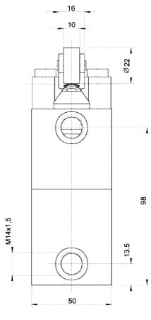
**3/2-Way-Valve Mechanically Operated** 3/2-way-valve, ND7, normally closed or normally open, 30 bar, M14 x 1.5, with pneumatic emergency operator
