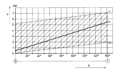
The characteristic line is infinitely adjustable in an parallel way within the shaded area and its gradient can be modified. Observe, that the pressure difference between initial and final pressure must be more than 1.85 bar. X) Handle travel, Y) Pressure in connection A
