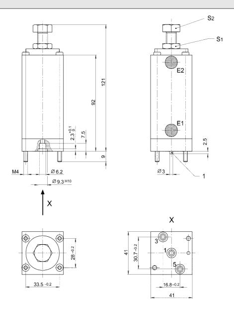
E) Exhaust, S1) Safety nut, S2) Adjusting screw, 1) Dowel pin
