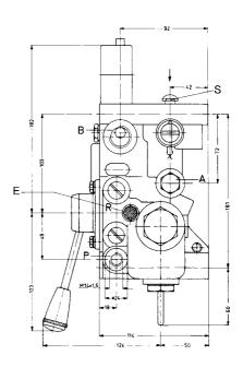
The device has to be mounted vertically as shown and will be fastened by two screws M 10 x 120.
