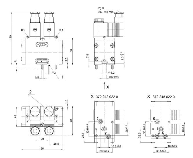
1) Dowel pin, 2) Check pin (extracted when respective solenoid is energized and if the pressure in connection 1> 4 bar)
