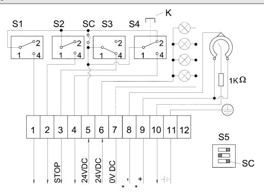
Speed increase / Gear interlock (warming-up function): by pressing button K and moving the lever over STOP in direction AHEAD or ASTERN the engine speed will be increased without engaging the clutch. When moving the lever back to STOP-position the gear function will be automatically active again. ATTENTION: Note switch C in the connection diagram! \*) Stabilized voltage
