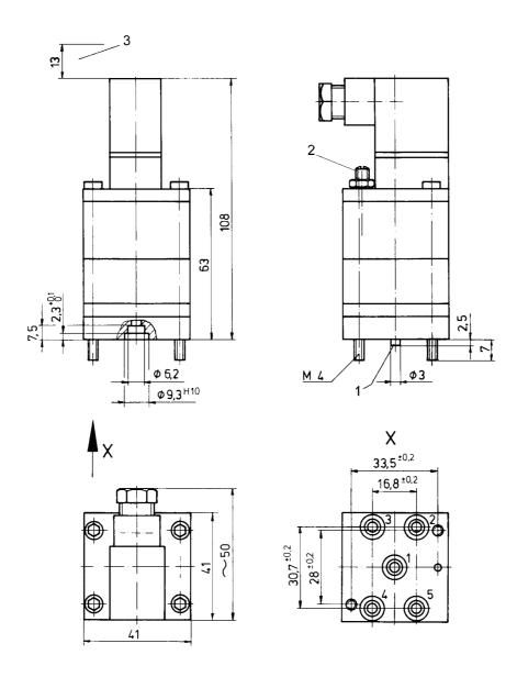
1) Dowel pin, 2) Adjusting screw for switching pressure, 3) Space to take out the connector
